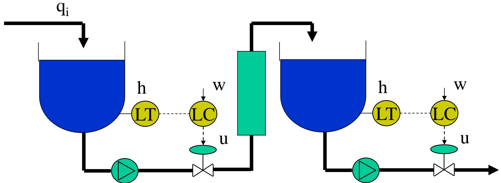
All level control must be placed in the same direction
