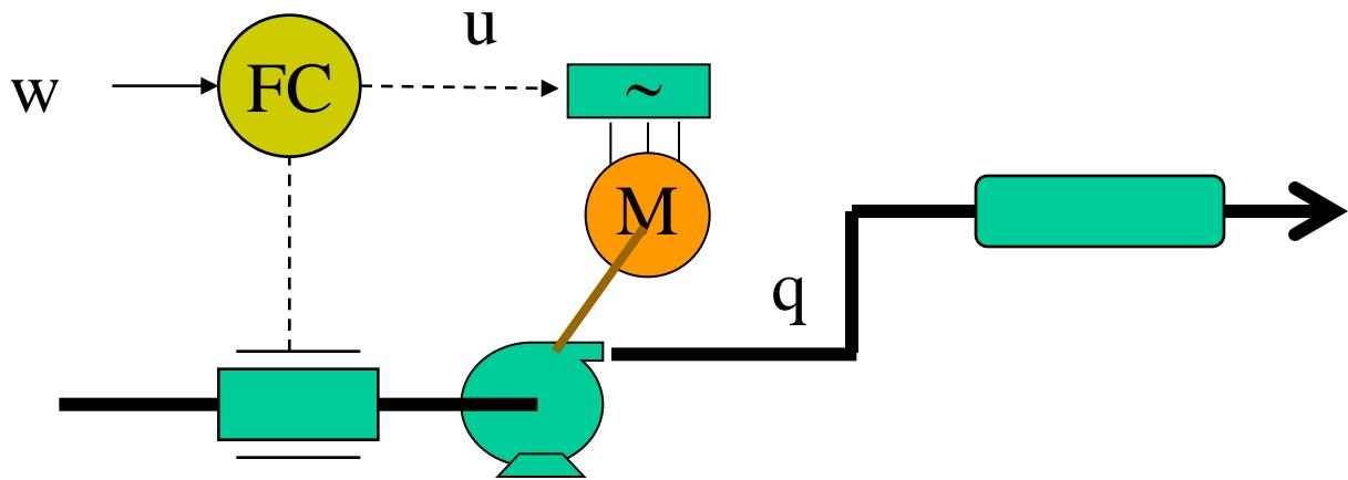
When the flow is high, instead of control valves, variable speed pumps are a sensible alternative that allows to save energy. A frequency converter (o similar device) connected to the pump asynchronous motor is required
