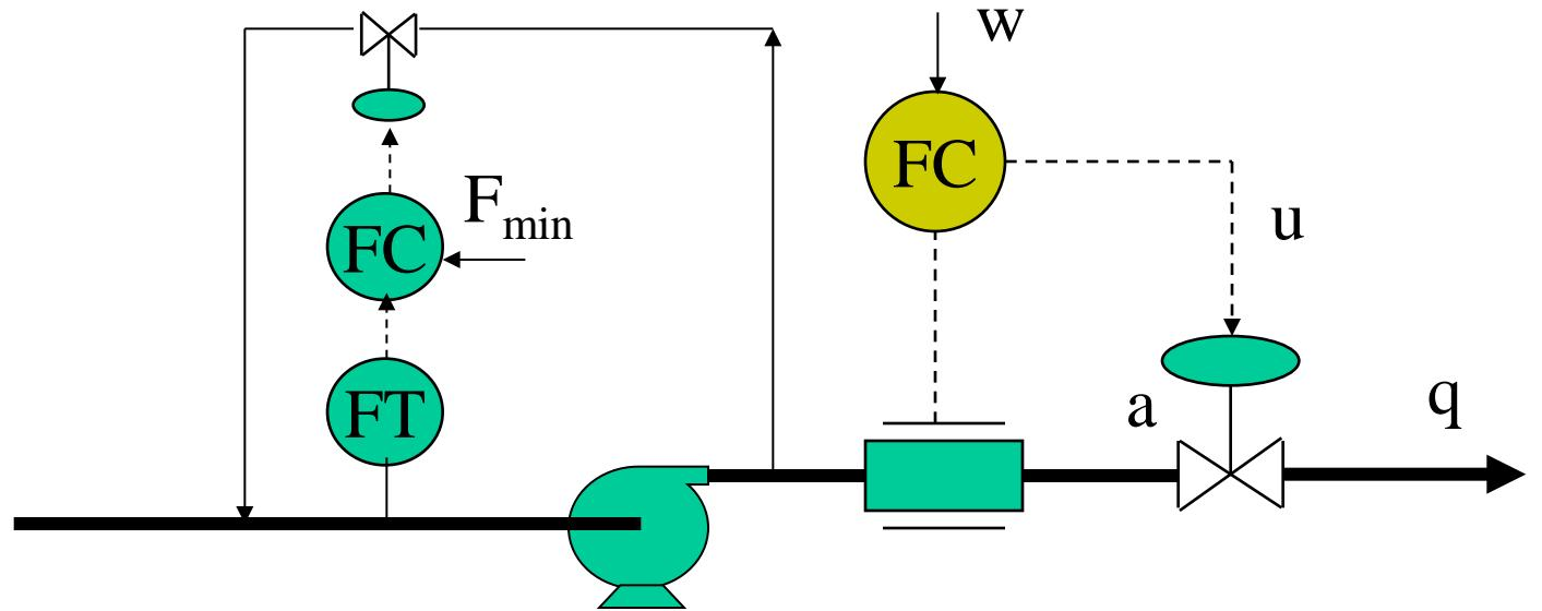
Sometimes, in order to guarantee a minimum flow through the pump, an extra flow loop is added. When  $w > F_{\min}$  the recirculation valve is closed, but if  $w < F_{\min}$  then the extra flow loop opens the recycle to maintain the required flow
