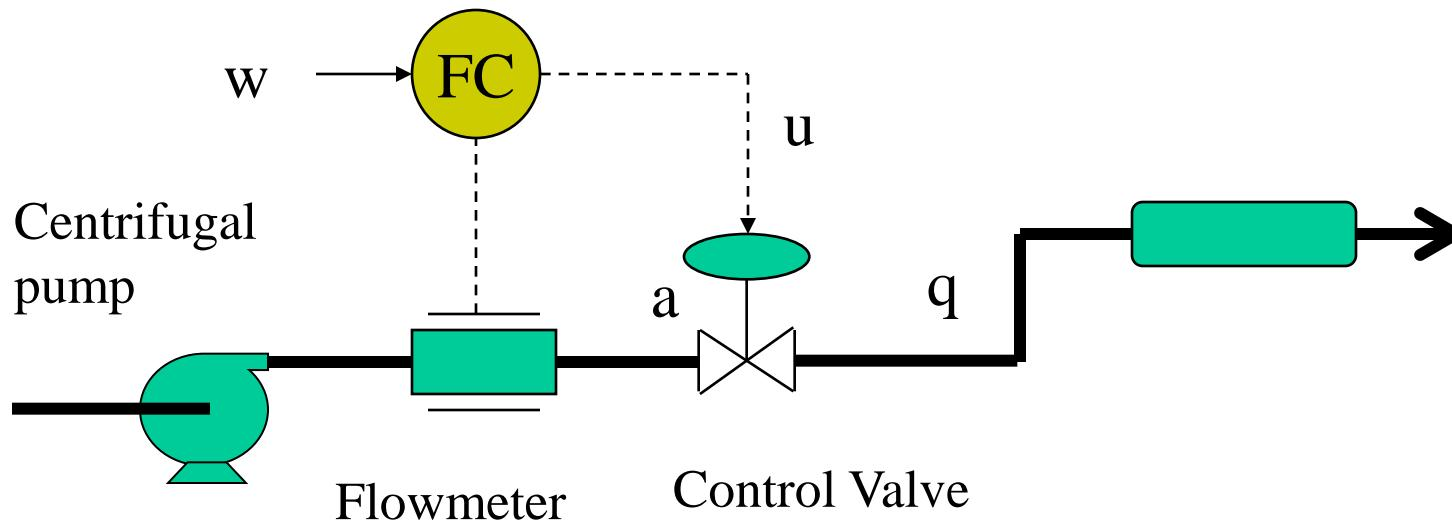
Pump, valve: sizing, placement
