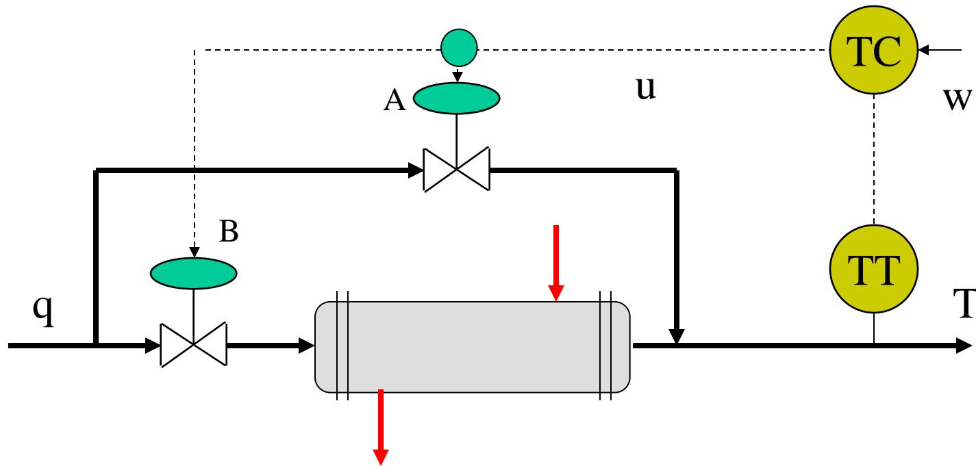
The valves operate in opposition, one is air-open and the other one air-close
