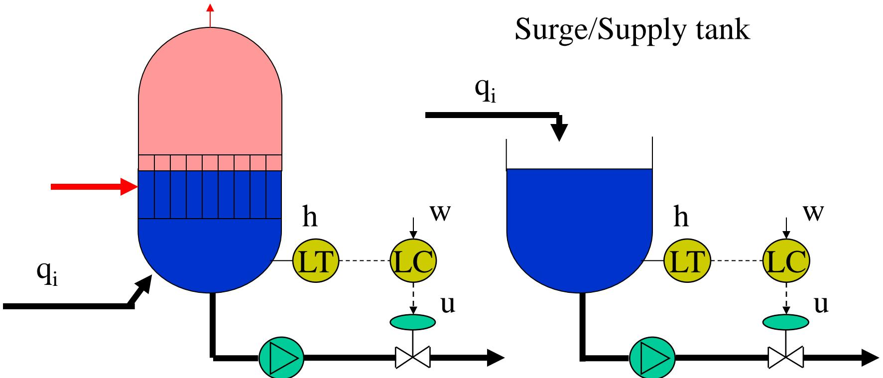
The level must be maintained tightly: PI with “active” tuning
