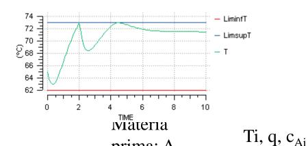
$V\rho c_{p} \frac{dT}{dt} = q\rho c_{p}(T_{i} - T) + Vkc_{A}H - UA(T - T_{r})$
