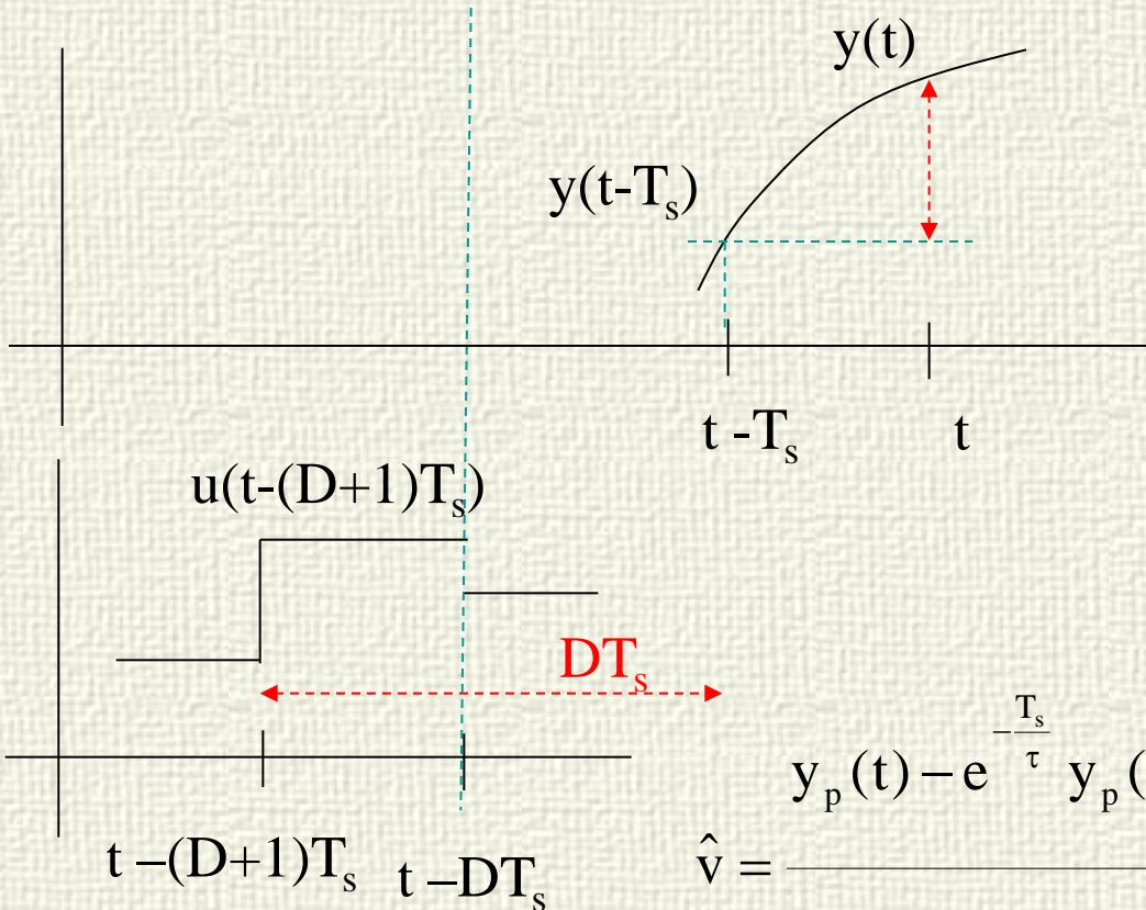
$v$  is estimated from the process model in order to cancel the difference between the measured process output at  $t$  and the prediction made with values at  $t - T_s$
