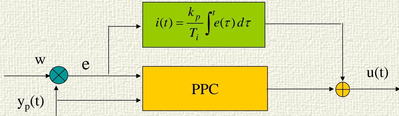
$$i(t) = i(t - T_s) + \frac{T_s}{T_i} e(t - T_s) = i(t - T_s) + \frac{T_s}{T_i} (w(t - T_s) - y_p(t - T_s))$$
