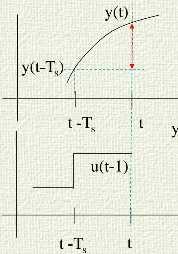
$v$  is estimated from the process model in order to cancel the difference between the measured process output at  $t$  and the prediction made with values at  $t - T_s$
