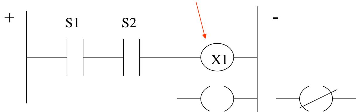
S1 or S2 can be any element providing a 0 – 1 signal: timers, counters, detectors, switches, etc.
