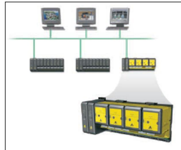
Per IEC 61508, the DeltaV SIS system and the DeltaV system are separate, yet have integrated engineering software.
