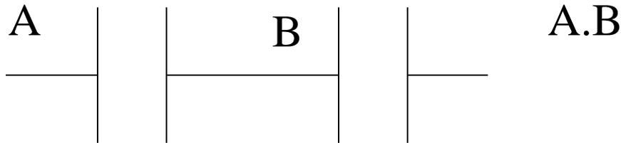
The light bulb is on if both, A and B, are closed
