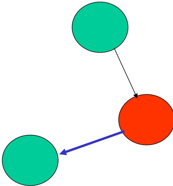
Transitions between states are formulated as logic functions of the system variables or time. A transition can be activated when the system is in the previous state and the logic condition is true. Each state have a set of associated actions.
