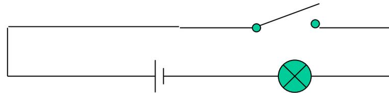
If the switch is closed, then the current flows through the circuit and the light bulb is activated
