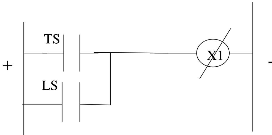
The steam input is stopped if the temperature or the level are out of limits 21
