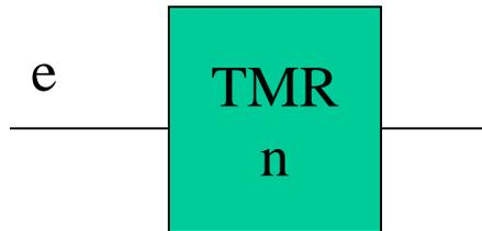
**Ton, Tof** Timer on/off Delay. The output is activated  $n$  time units after the input is activated. The timer is reset if the input does not keep active for  $n$  seconds
