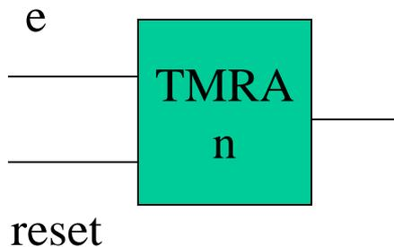
The output is activated  $n$  time units after the input is activated. If  $e$  is deactivated before  $n$ , the timer keep the accumulated time. The timer is reset only if the reset signal is activated
