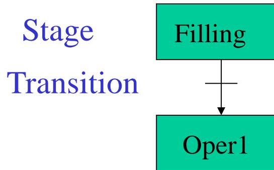
When the logic condition associated to a transition becomes true (and the process is in the corresponding stage), the current stage is deactivated and the following one is activated, besides executing all its associated actions. The logic condition can be formulated in any of the IEC 61131 languages
