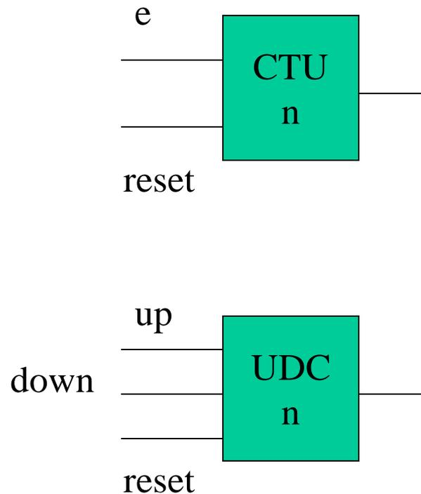
The output is activated when the input changes from false to true  $n$  times. The counter is reset to zero when the reset input is activated.
