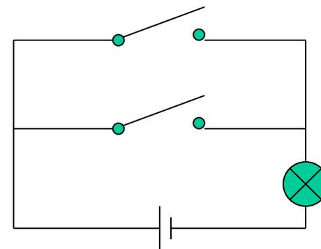
The light bulb is on if any, A or B, is closed
