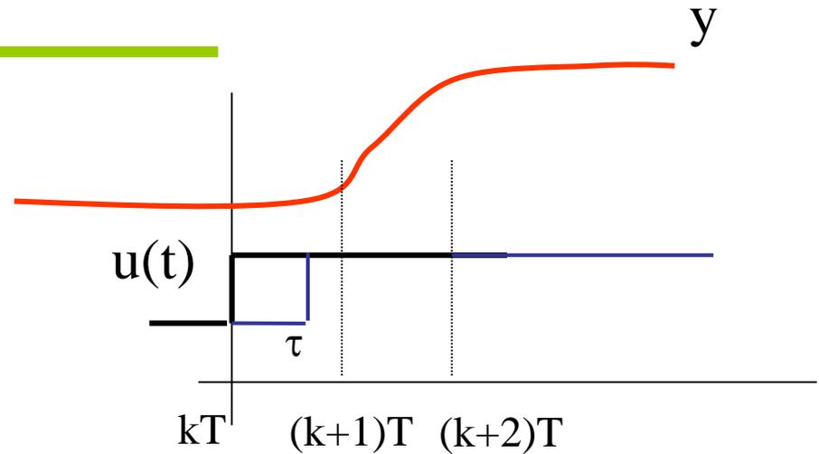
$$\begin{aligned} x((k+1)T) &= e^{AT} x(kT) + \int_{kT}^{(k+1)T} e^{A((k+1)T-\sigma)} Bu(\sigma - \tau) d\sigma = \\ &= e^{AT} x(kT) + \int_{kT}^{kT+\tau} e^{A((k+1)T-\sigma)} d\sigma Bu((k-1)T) + \\ &+ \int_{kT+\tau}^{(k+1)T} e^{A((k+1)T-\sigma)} d\sigma Bu(kT) \end{aligned}$$
