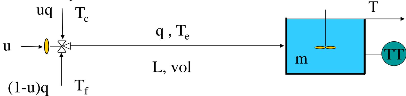
$$q\rho c_e T_e(t) = u(t)q\rho c_e T_c + (1 - u(t))q\rho c_e T_f \Rightarrow T_e(t) = u(t)T_c + (1 - u(t))T_f$$
