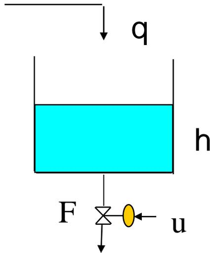
$$\frac{d\Delta h}{dt} = -\frac{u_0 k}{2A\sqrt{h_0}} \Delta h - \frac{k\sqrt{h_0}}{A} \Delta u + \frac{1}{A} \Delta q$$
