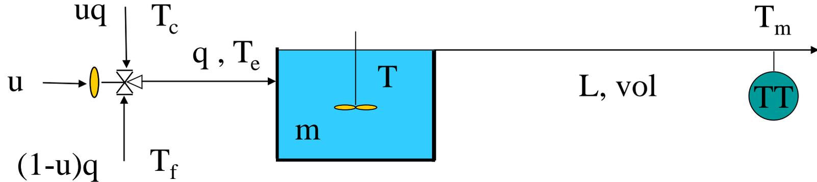
$$\frac{V}{q} \frac{d \Delta T(t)}{dt} + \Delta T(t) = (T_c - T_f) \Delta u(t) \quad \Delta T_m(t + \tau) = \Delta T(t)$$
