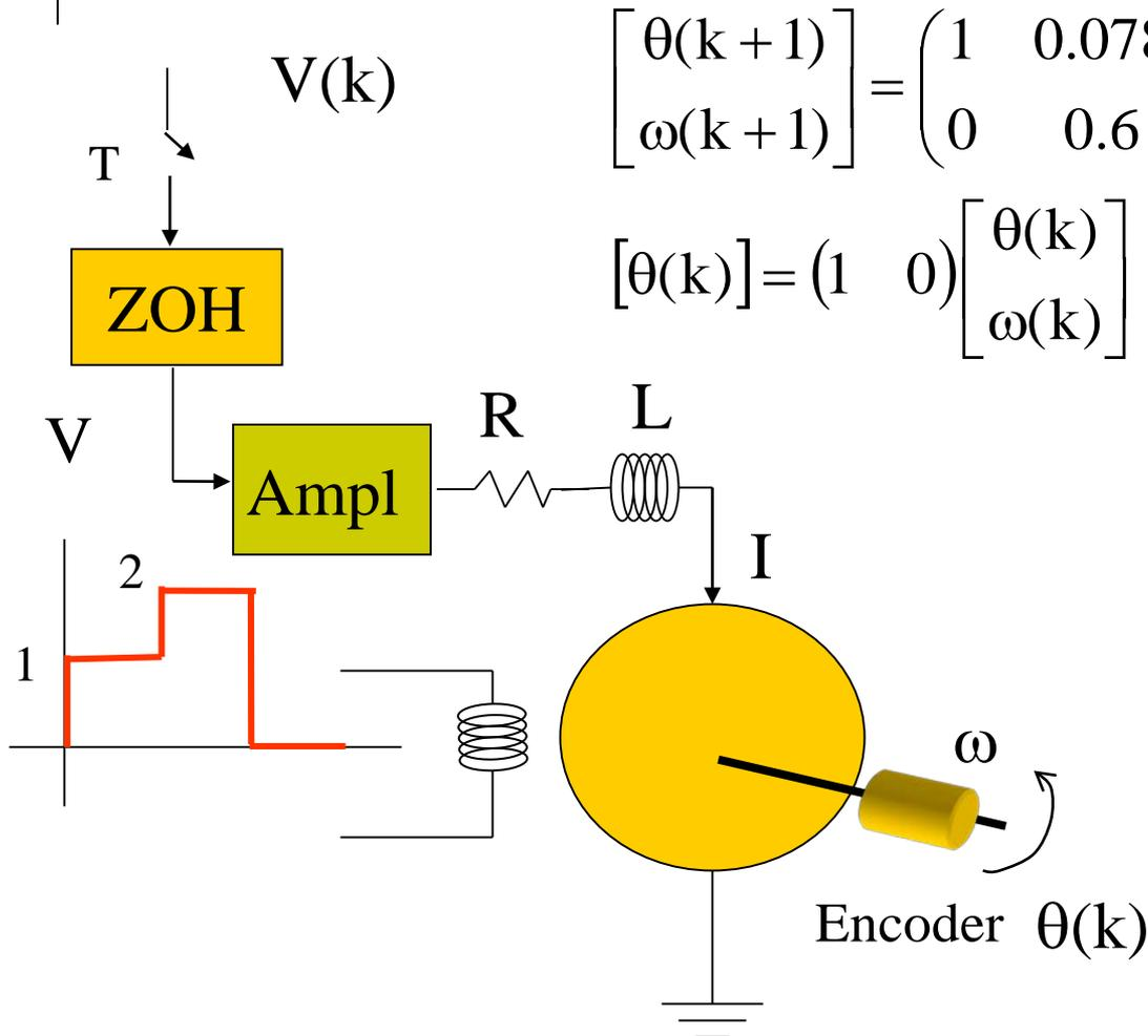
$$\begin{bmatrix} \theta(k+1) \\ \omega(k+1) \end{bmatrix} = \begin{pmatrix} 1 & 0.078 \\ 0 & 0.6 \end{pmatrix} \begin{bmatrix} \theta(k) \\ \omega(k) \end{bmatrix} + \begin{pmatrix} 2.123 \\ 39.154 \end{pmatrix} V(k)$$
