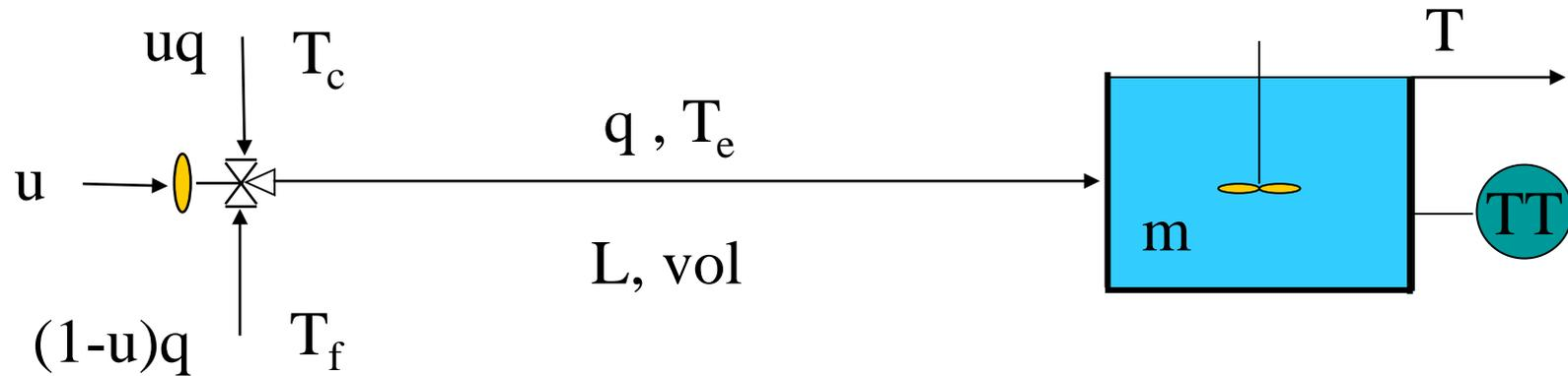
$$\frac{V}{q} \frac{d \Delta T(t)}{dt} + \Delta T(t) = (T_c - T_f) \Delta u(t - \tau) \Rightarrow T(s) = \frac{e^{-\tau s} (T_c - T_f)}{\frac{V}{q} s + 1} U(s)$$
